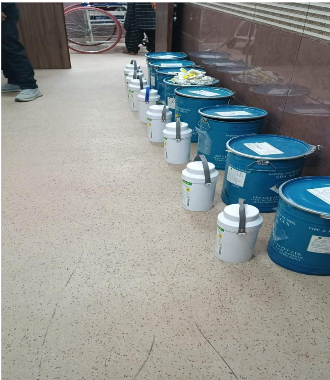
Radioactive waste containers
