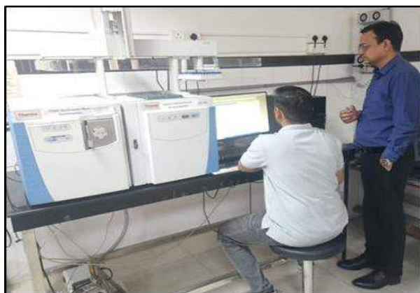
Figure 3: GC-MS/MS equipment analyzing metabolites and pesticides in various biological samples
