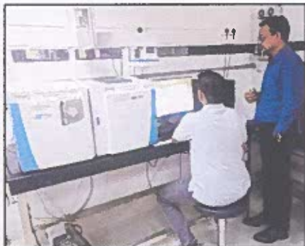
Figure 3: GC-MS/MS equipment analysing metabolites and pesticides in various biological samples.
